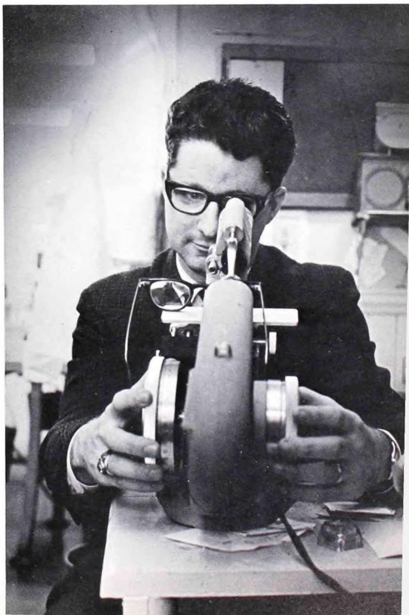
The accuracy of the finished job is checked by Clinician P. Heyman by careful use of the vertometer.
