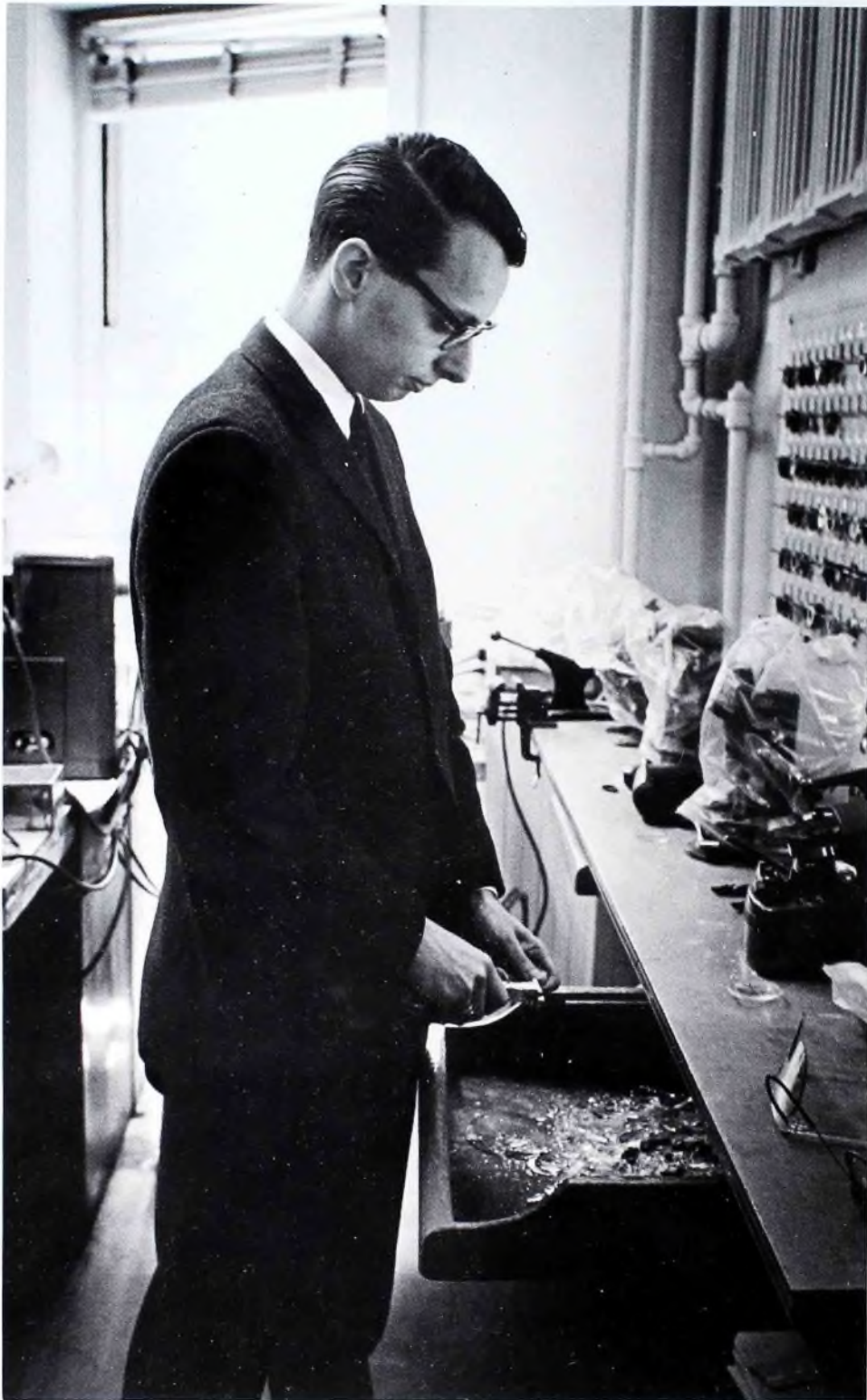
Before placing the lens in the automatic beveling machine behind him, Clinician J. Abraham removes excess glass from the cut lens blank.
