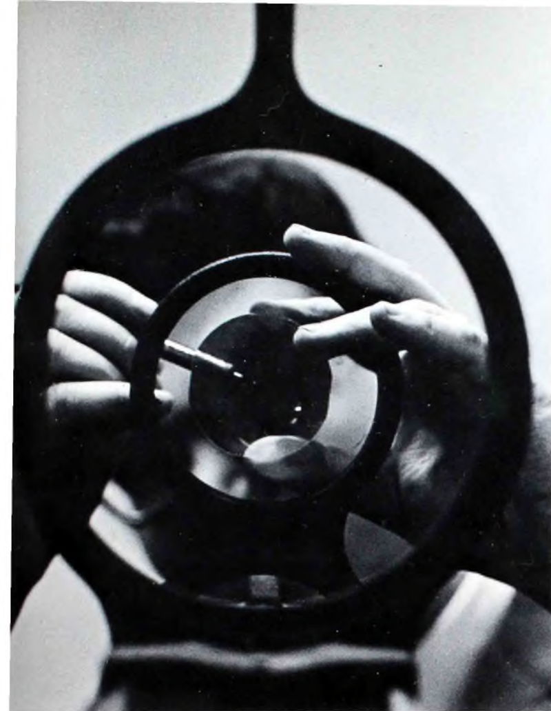
A sighting device is used to correctly line up an uncut lens blank.
