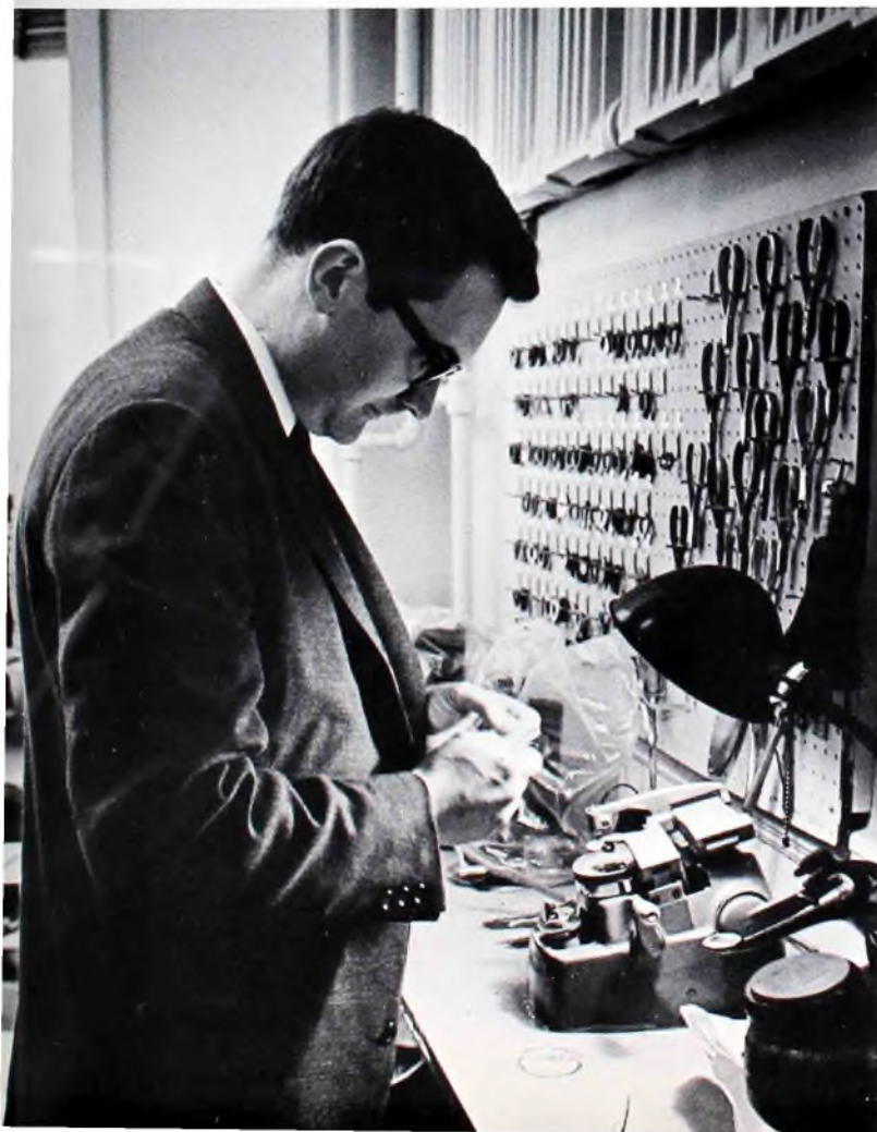
Clinician T. Edmonds prepares to cut the lens blank to the appropriate shape for the selected frame.
